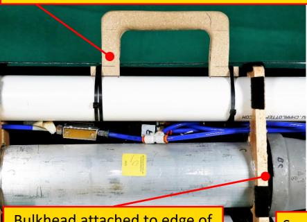
Bulkhead attached to edge of tank reducer with Velcro
