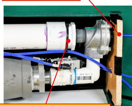
Secure Line from Air Tanks here to Avoid Pulling on Quick Connect
