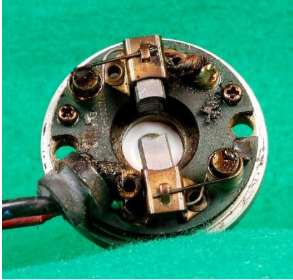
Brush Card Construction Similar to CIM Motors
