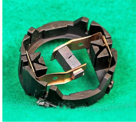
Connector and cantilever spring are one part
